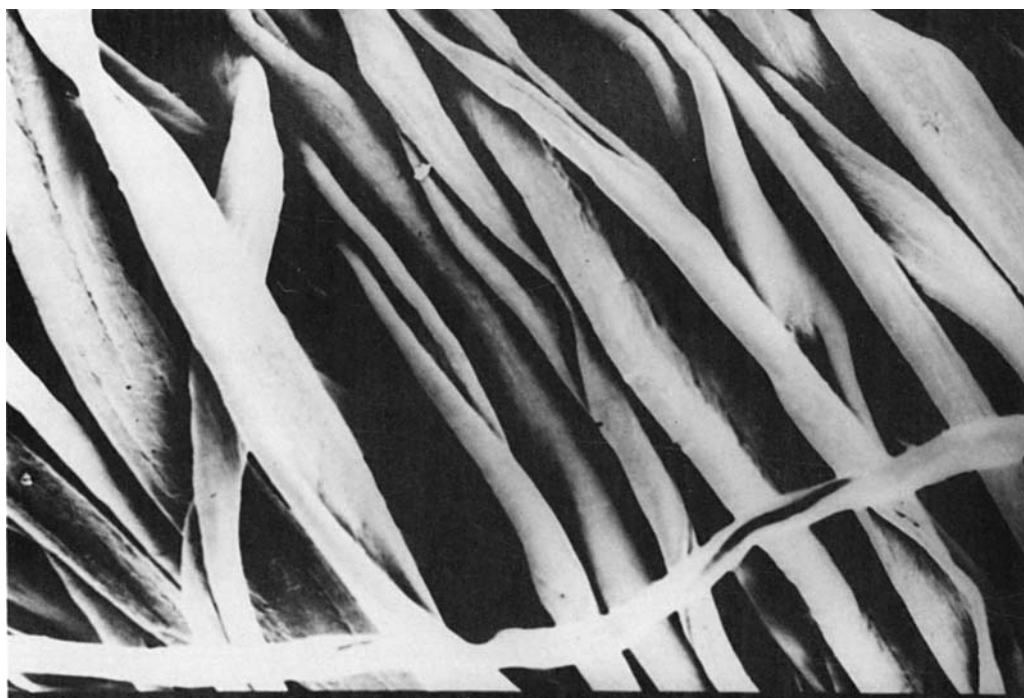
Figure 1 Scanning electron micrograph of scoured, ZnCl_2 - and NaOH-treated yarns: scoured open end yarn.
